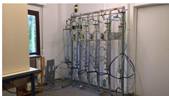
Figure 1. Laboratory gas mixing and parallel reactor arrangement used for comparative H_2S breakthrough testing; similar to ASTM D6646 accelerated breakthrough testing (Courtesy of Hego Biotec International GmbH).
